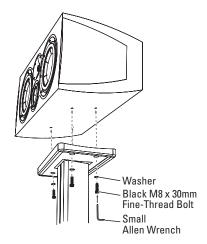
IMPORTANT: If you are attaching the C208 or C205 to the C-Stand you cannot use the adjustable feet that were included with the speaker. The C-Stand places the speaker at the proper angle for seated listeners without requiring additional adjustments.
